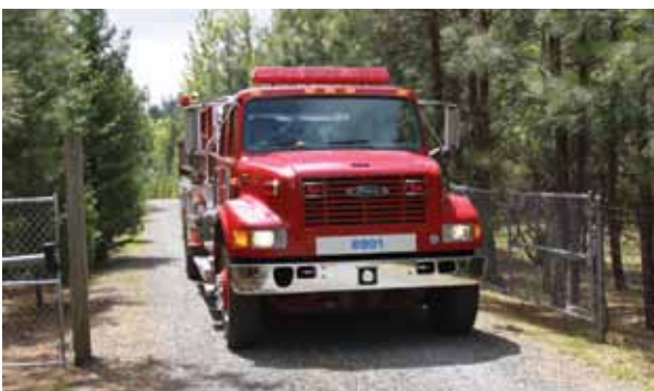
Don't make fire trucks stop at the gate. A gate needs to be 14 feet wide on straight roads and 16 feet wide on curves.
